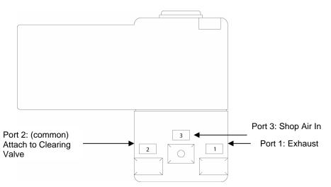
Figure 29: Clearing Valve Compressed Air Connections
